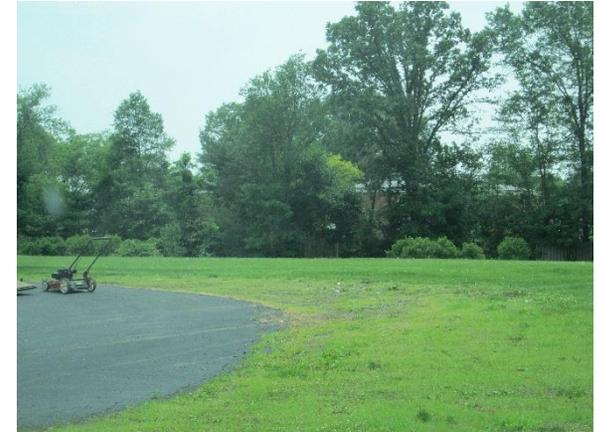
In the back parking lot there is evidence of erosion in the turf grass. A bioretention system can be installed in this area along the curve of the driveway to capture, treat, and infiltrate stormwater runoff. A preliminary soil assessment suggests that more soil testing would be required before determining the soil's suitability for green infrastructure.
